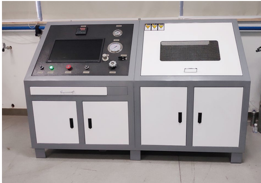
Pressure and leak test equipment
