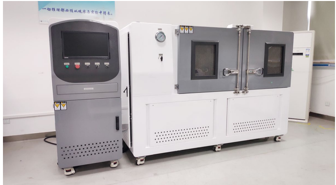
Flow-pressure test equipment
