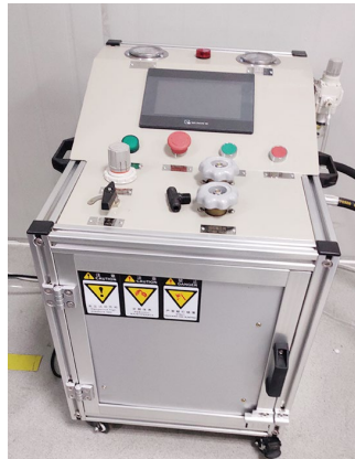
Air tightness test equipment
